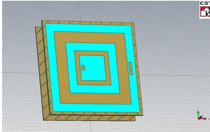
The simulated model respects the geometrical characteristics reported in *Tab. I*. For ground plane substrate the thickness has been set to 0.8 mm.
