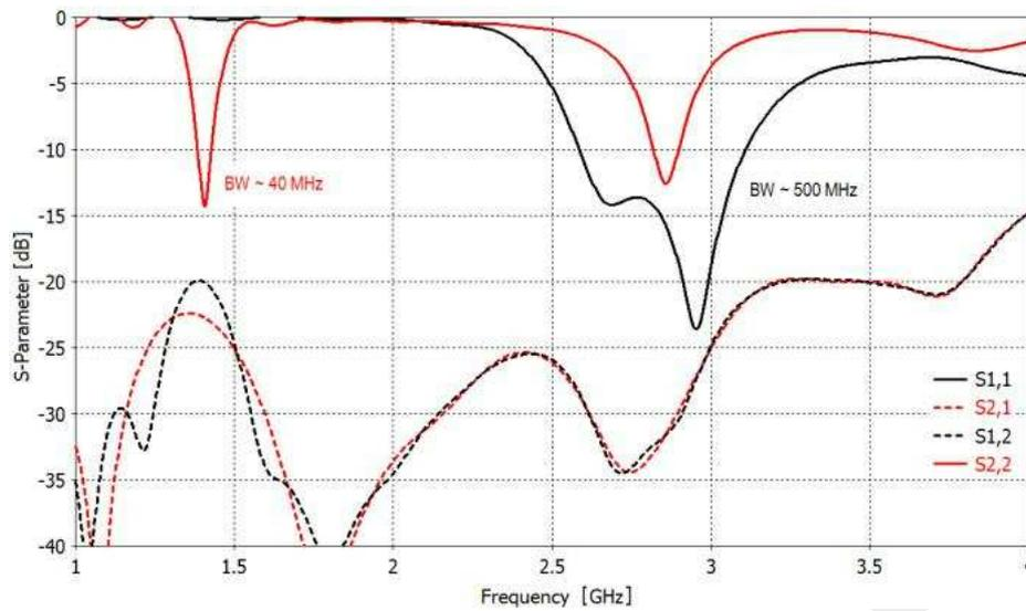
Figure 2: Reflection coefficients for L-band and S-band
