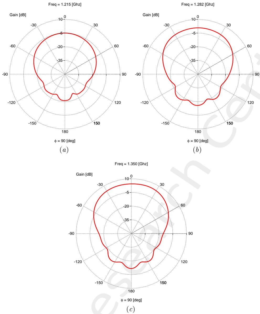
Figure 11: 2D Embedded Element Gain Pattern for  $\phi = 90$ [deg]: (a)  $f = 1.215$  GHz, (b)  $f = 1.282$  GHz, (c)  $f = 1.350$  GHz
