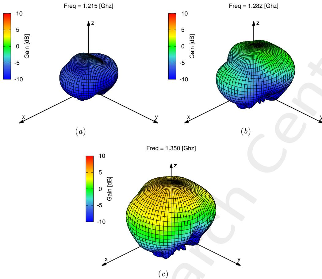
Figure 9: 3D Embedded Element Gain Pattern for: (a)  $f = 1.215$  GHz, (b)  $f = 1.282$  GHz, (c)  $f = 1.350$  GHz
