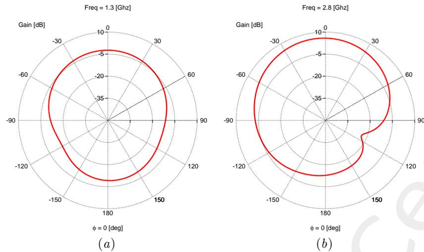
Figure 5: 2D Antenna Gain Pattern for  $\phi = 0[\text{deg}]$ : (a) L-band  $f = 1.3 \text{ GHz}$ , (b) S-band  $f = 2.8 \text{ GHz}$
