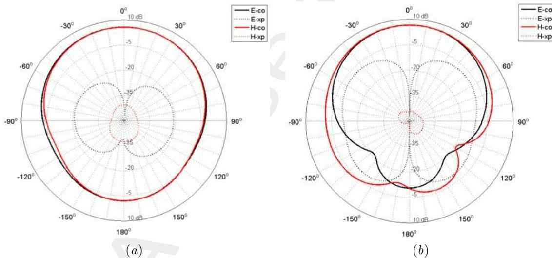
Figure 3: Power patterns for L-band (a) and S-band (b)
