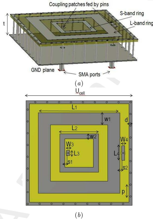
Figure 1: Radiating element, 3D view (a), top view (b)
