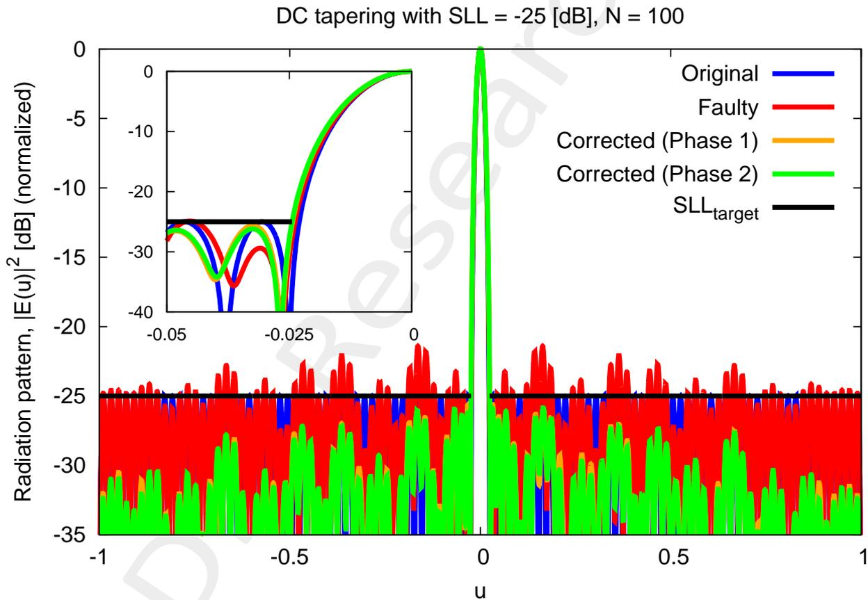
Figure 9: The radiation pattern for the original, faulty and corrected excitations for the array with 100 elements. The smaller rectangle within the figure shows the peak side lobe of the faulty-state pattern being suppressed in the corrected pattern.
