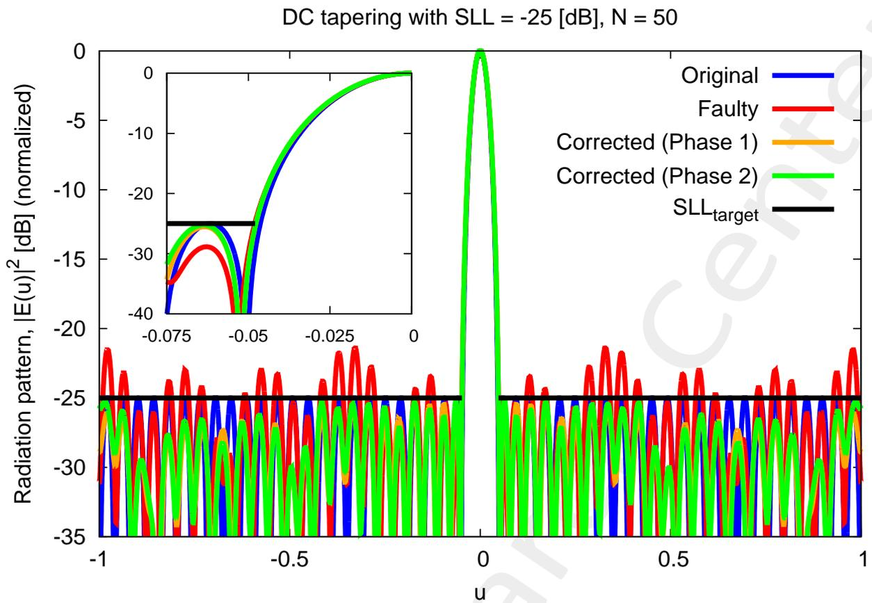
Figure 6: The radiation pattern for the original, faulty and corrected excitations for the array with 50 elements. The smaller rectangle within the figure shows the peak side lobe of the faulty-state pattern being suppressed in the corrected pattern.
