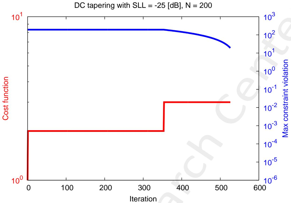
Figure 16: The value of the L1-norm cost function for each iteration of the algorithm for the array with 200 elements.
