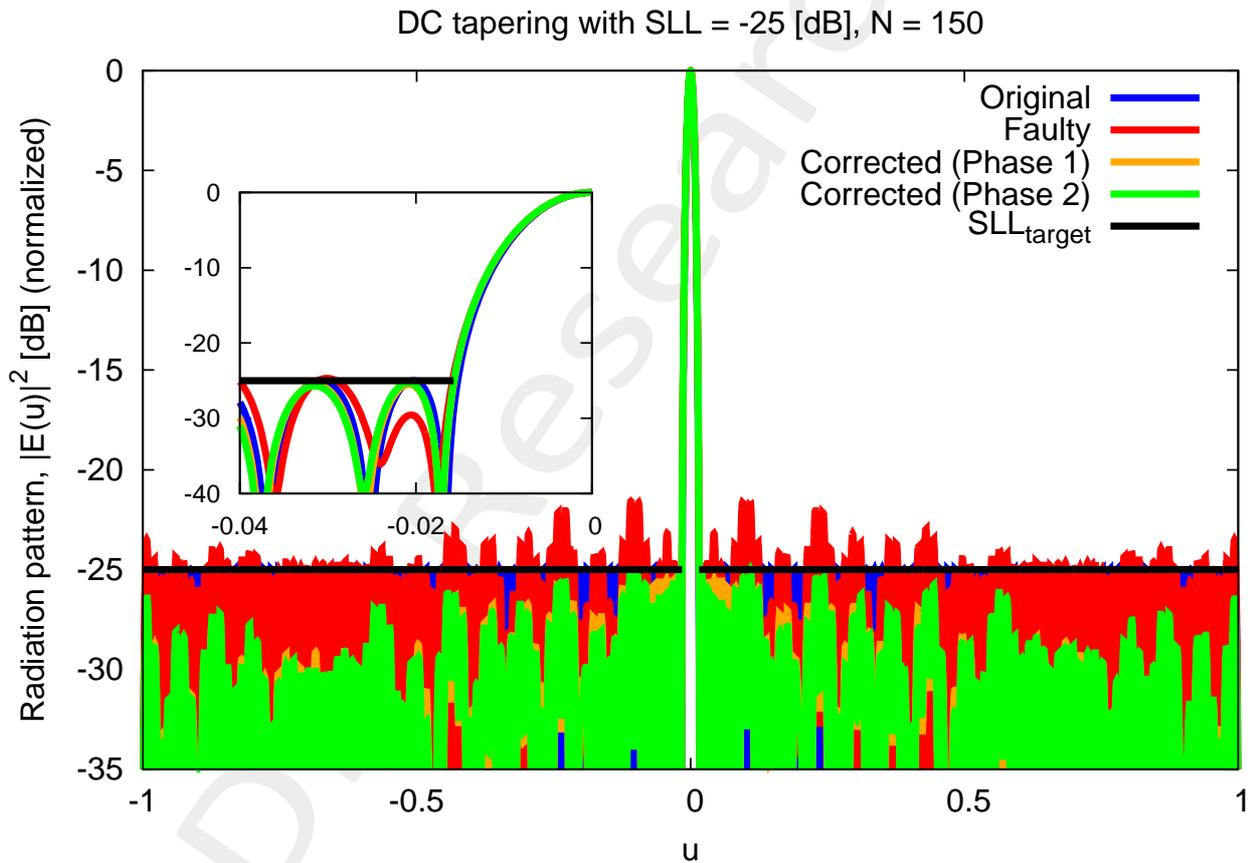
Figure 12: The radiation pattern for the original, faulty and corrected excitations for the array with 150 elements. The smaller rectangle within the figure shows the peak side lobe of the faulty-state pattern being suppressed in the corrected pattern.
