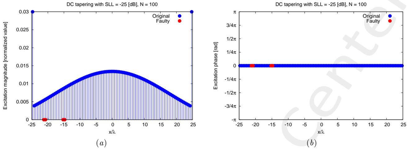
Figure 2: Original and damaged excitations for the array with  $N = 100$  elements considered in test case 5: amplitude (a) and phase (b).
