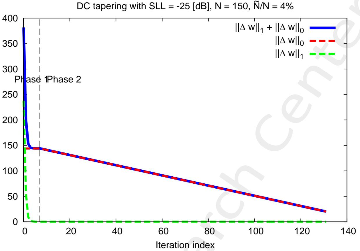
Figure 13: The value of the L1-norm cost function for each iteration of the algorithm for the array with 150 elements.
