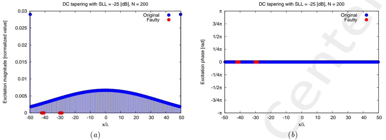
Figure 4: Original and damaged excitations for the array with  $N = 200$  elements considered in test case 5: amplitude (a) and phase (b).
