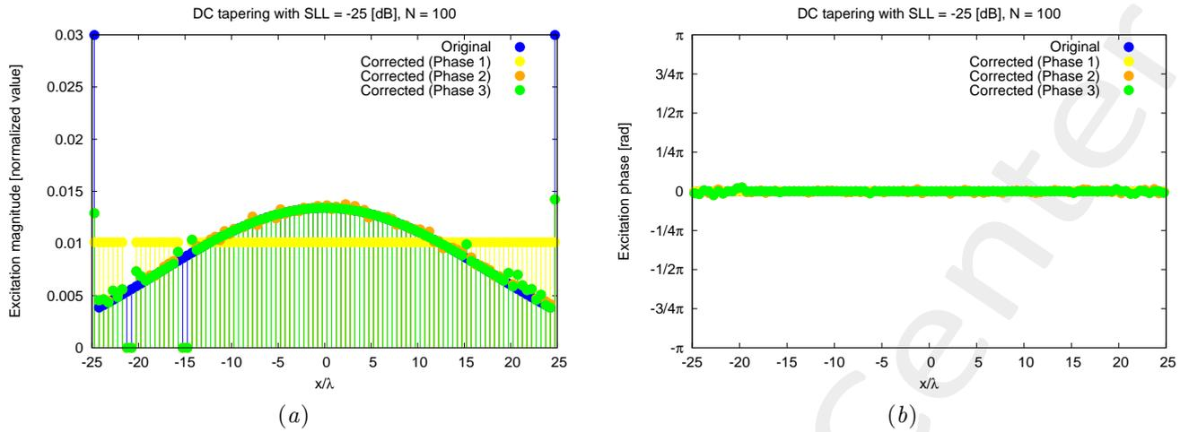
Figure 11: Original and corrected excitations for the array with 150 elements: amplitude (a) and phase (b).
