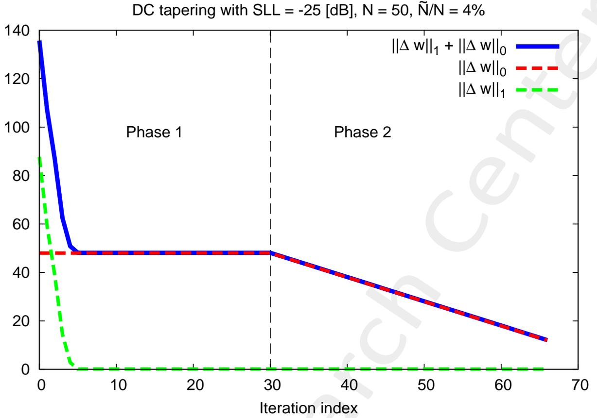
Figure 7: The value of the L1-norm cost function for each iteration of the algorithm for the array with 50 elements.
