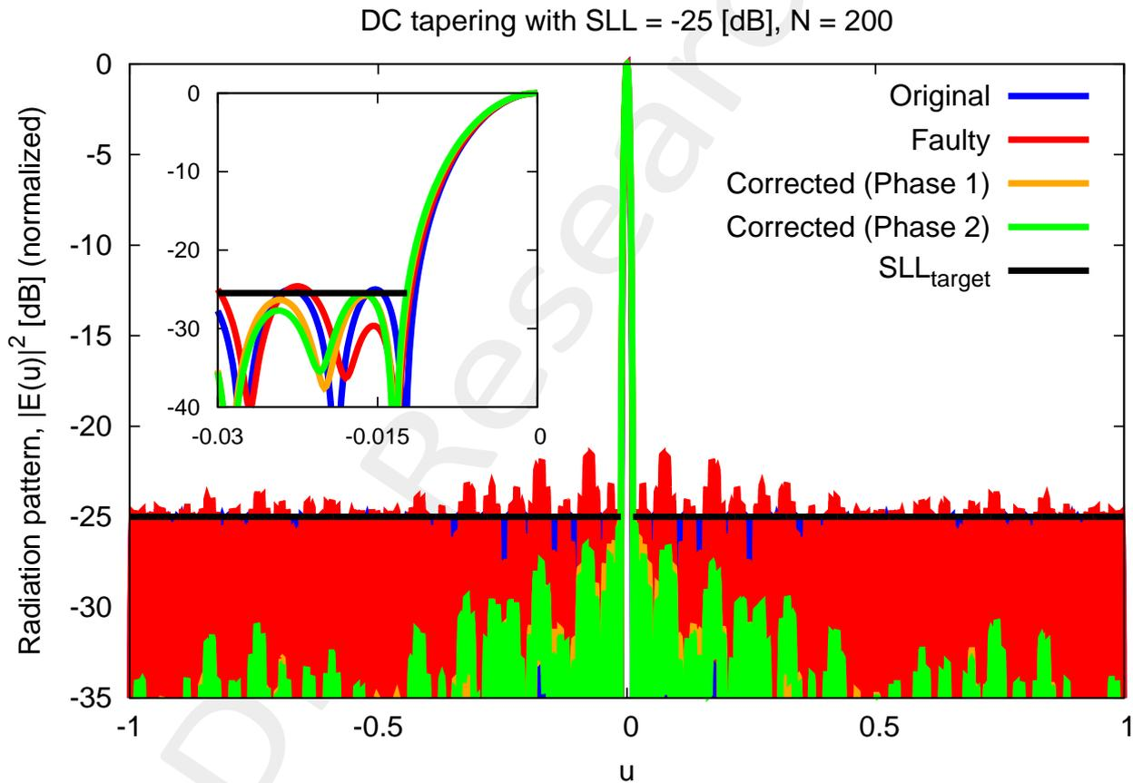
Figure 15: The radiation pattern for the original, faulty and corrected excitations for the array with 200 elements. The smaller rectangle within the figure shows the peak side lobe of the faulty-state pattern being suppressed in the corrected pattern.
