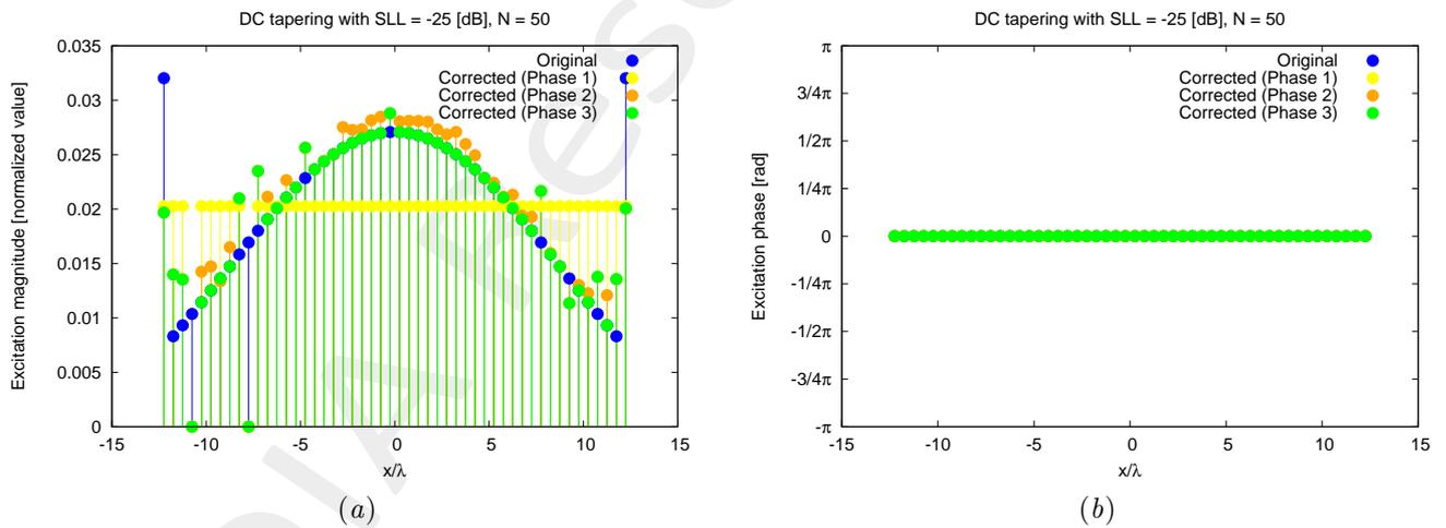
Figure 5: Original and corrected excitations for the array with 50 elements: amplitude (a) and phase (b).
