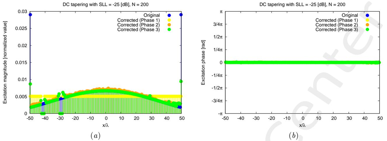
Figure 14: Original and corrected excitations for the array with 200 elements: amplitude (a) and phase (b).
