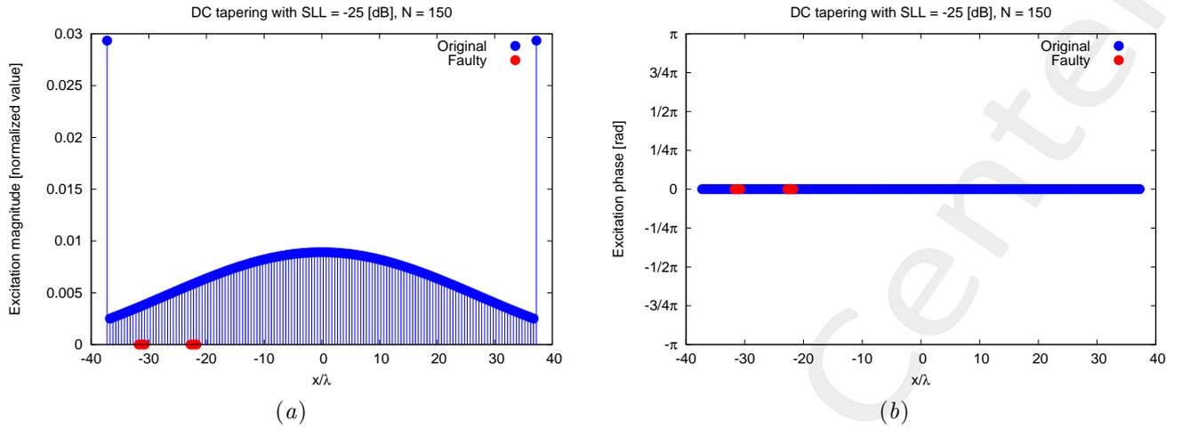
Figure 3: Original and damaged excitations for the array with  $N = 150$  elements considered in test case 5: amplitude (a) and phase (b).
