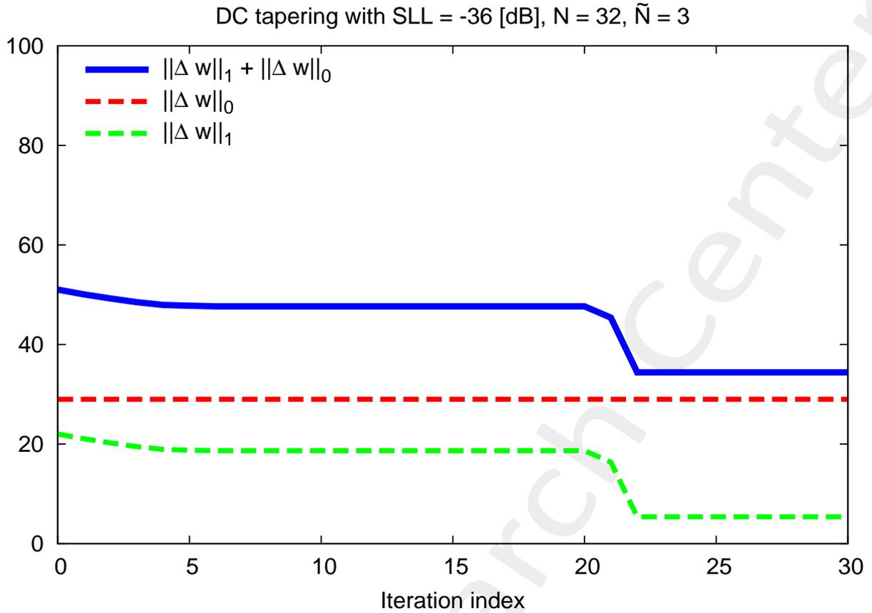
Figure 9: The value of the L1-norm cost function for each iteration of the algorithm.
