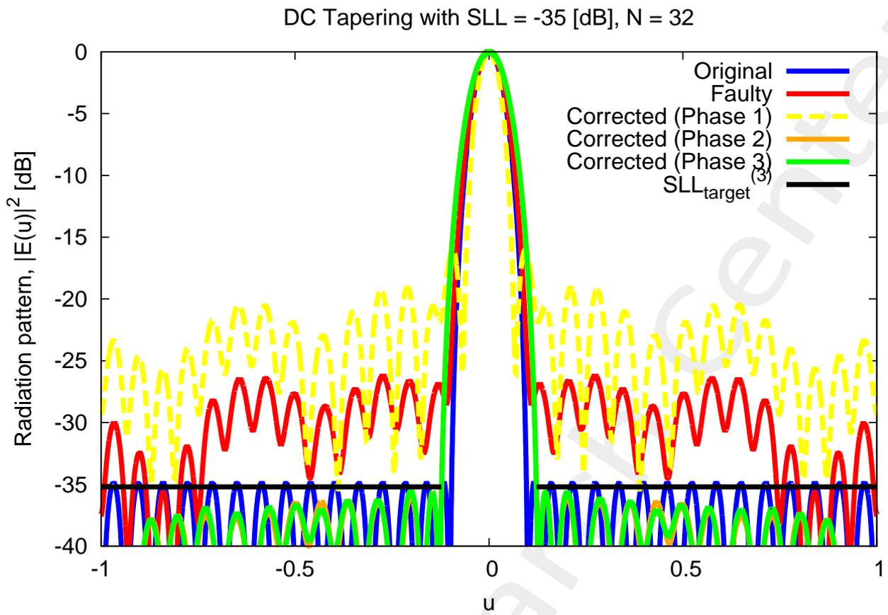
Figure 8: The radiation pattern for the original, faulty and corrected excitations.
