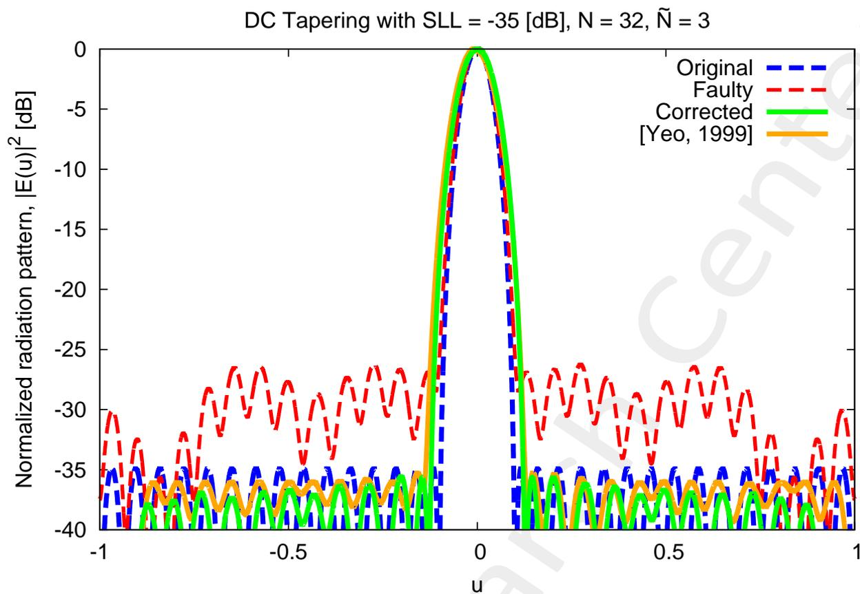
Figure 10: The corrected patterns obtained with the proposed and reference methods are shown, along with the original and faulty patterns.
