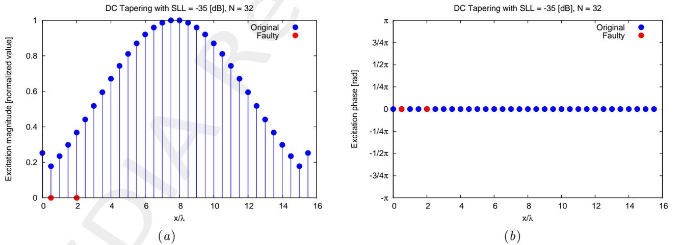
Figure 1: Original and damaged excitations for the array considered in test case 3: amplitude (a) and phase (b).
