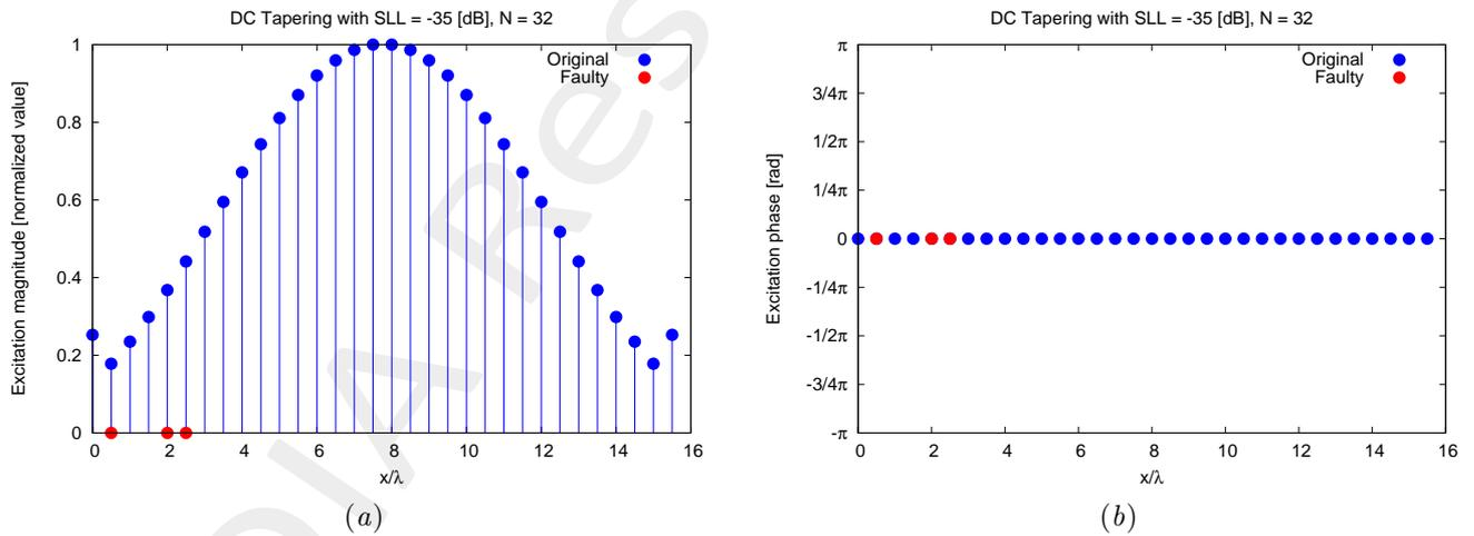
Figure 6: Original and damaged excitations for the array considered in test case 4: amplitude (a) and phase (b).
