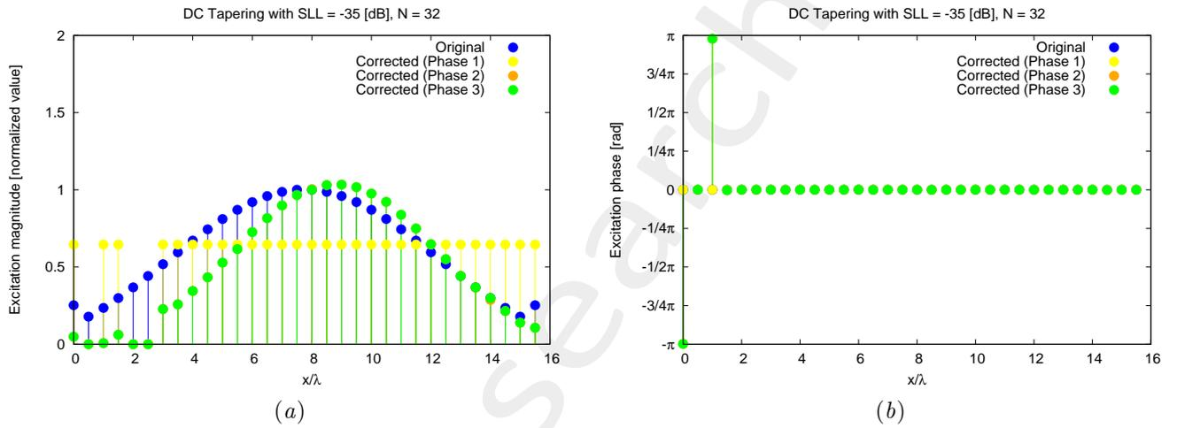
Figure 7: Original and corrected excitations for the array considered in test case 1: amplitude (a) and phase (b).
