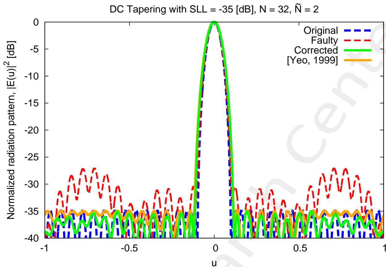
Figure 5: The corrected patterns obtained with the proposed and reference methods are shown, along with the original and faulty patterns.
