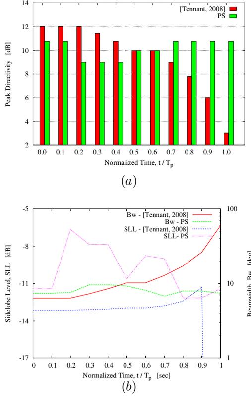
Fig. 3. Experiment 1 ( $N = 16, d = 0.5\lambda$ ) - Values of (a)  $D_{max}$  and of (b) SLL and BW for the DC solution and the solution obtained by means of the PS technique when sampling the current distribution on the array aperture at each tenth of the modulation period  $T_p$ .
