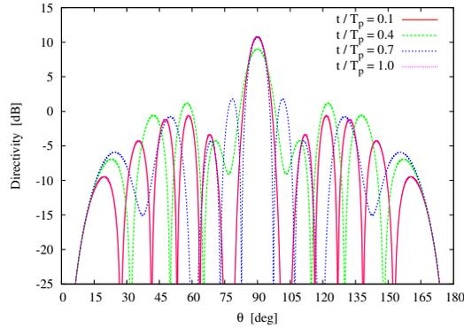
Fig. 2. *Experiment 1* ( $N = 16, d = 0.5\lambda$ ) - Plots of the directivity patterns obtained at the carrier frequency when sampling the current distribution on the array aperture at  $\frac{t}{T_p} = \{0.1, 0.4, 0.7, 1.0\}$  for the solution obtained by means of the *PS* technique.
