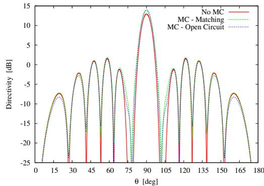
Fig. 4. Experiment 1 ( $N = 16, d = 0.5\lambda$ ) - Directivity patterns obtained for a dipole array with and without mutual coupling at  $\frac{t}{T_p} = 0.1$ .
