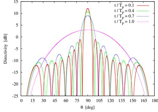
Fig. 1. *Experiment 1* ( $N = 16, d = 0.5\lambda$ ) - Plots of the directivity patterns obtained at the carrier frequency when sampling the current distribution on the array aperture at  $\frac{t}{T_p} = \{0.1, 0.4, 0.7, 1.0\}$  for the *DC* solution.
