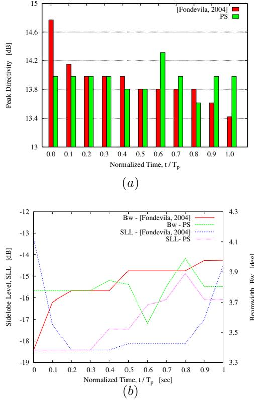
Fig. 5. Experiment 2 ( $N = 30$ ,  $d = 0.7\lambda$ ) - Values of (a)  $D_{max}$  and of (b) SLL and BW for the DC solution and the solution obtained by means of the PS technique when sampling the current distribution on the array aperture at each tenth of the modulation period  $T_p$ .
