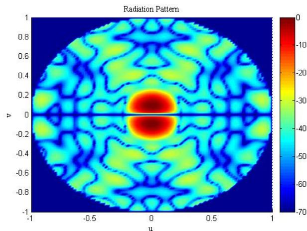
Figure 4: sub-arrayed E difference mode – dB scale
