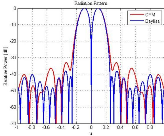
Figure 5: H-mode for  $v=0$  – Optimal and Subarrayed Pattern
