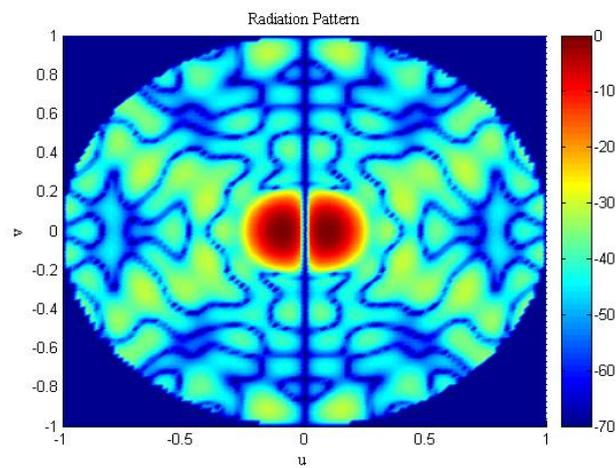
Figure 3: sub-arrayed H difference mode – dB scale
