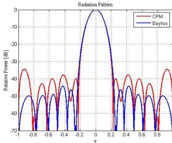
Figure 6: H-mode for  $u=0$  – Optimal and Subarrayed Pattern
