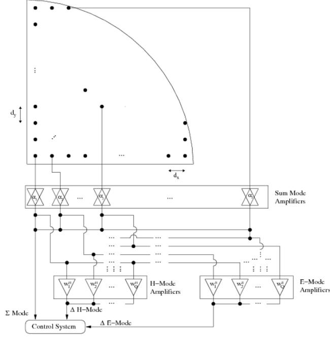
Figure 1: Sub-arrayed antenna feed network
