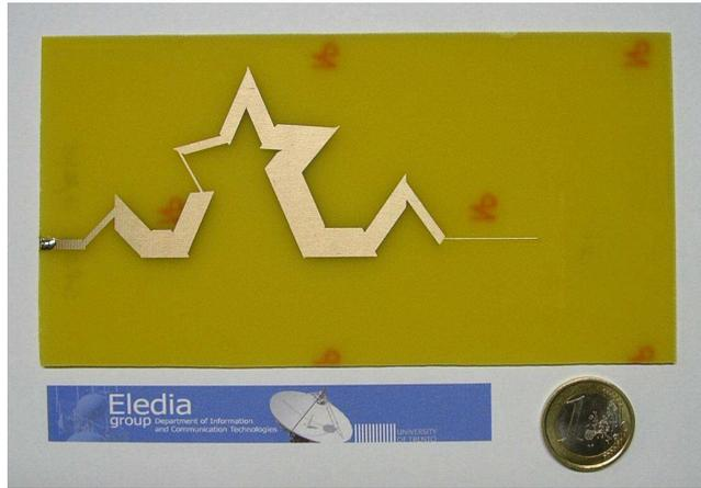
Figure 5 - R. Azaro *et al.*, “Synthesis of a pre-fractal dual-band monopolar ...”
