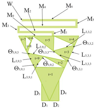
Fig. 1. Geometry of the reference antenna shape.
