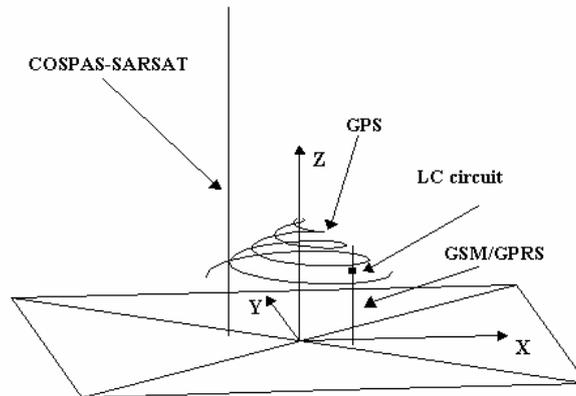
**Figure 1.** Geometry of the integrated multi-function antenna
