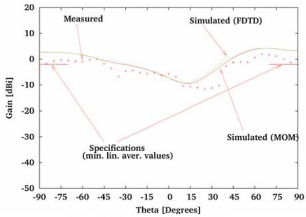
(c) GSM/GPRS upper band (1850 MHz)
