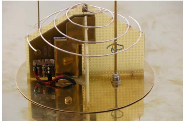
**Figure 2.** A photograph of the integrated multi-function antenna
