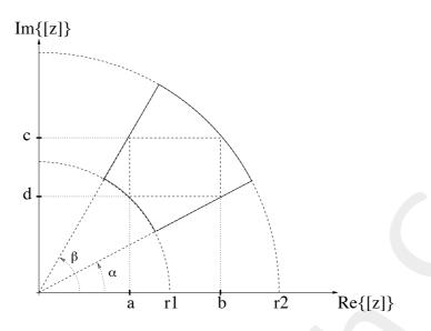
**Figure 2.3.2:** Complex interval in cartesian and polar form,  $[z] = [a, b] + j \cdot [c, d]$  or  $[z] = [r_1, r_2] \cdot e^{j \cdot [\alpha, \beta]}$ .
