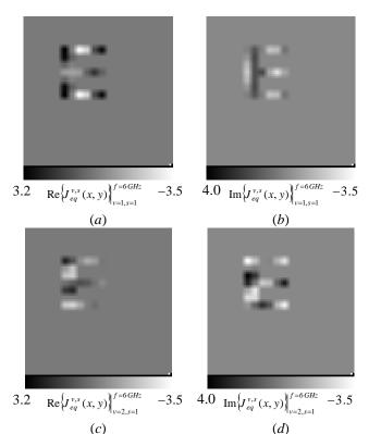
Fig. 2. Equivalent current distribution induced in the investigation domain by a plane illumination (s = 1) at f = 6 GHz: Real (a) and Imaginary part (b) when (v = 1). Real (c) and Imaginary part (d) when (v = 2).
