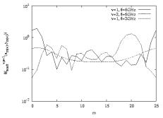
Fig. 3. Amplitude of the scattered field collected in  $D_o$  under plane wave (s = 1) illumination for different views and frequencies.
