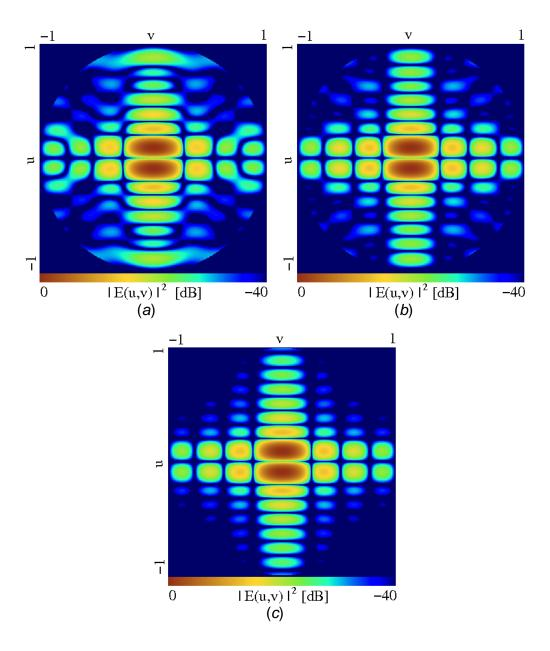
Fig. 3 - E-mode difference pattern: (a) compromise with Q=4, (b) compromise with Q=8, and (c) reference.
