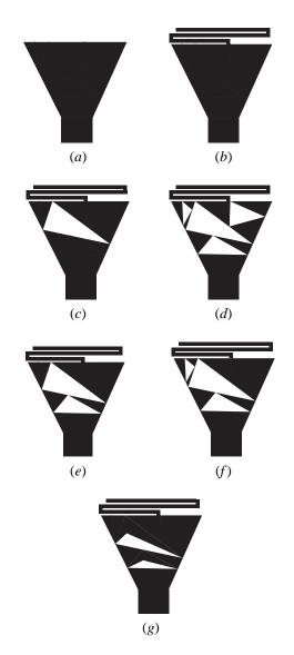
Fig. 4. Three-band hybrid prefractal antenna - Intermediate geometries.
