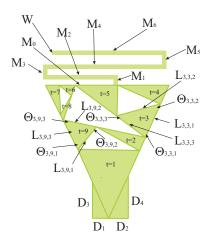
Fig. 1. Geometry of the reference antenna shape.
