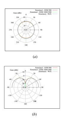
Fig. 6. Three-band hybrid prefractal antenna - Behavior of the gain function along the horizontal plane  $[(a) - \theta = 90^{\circ}]$  and the vertical plane  $[(b) - \phi = 0^{\circ}]$ , respectively.
