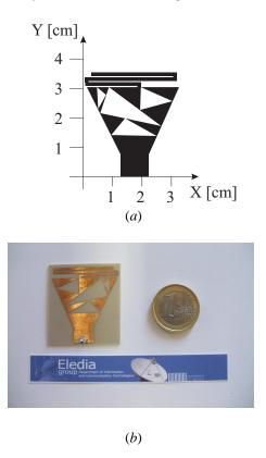
Fig. 2. *Three-band hybrid prefractal antenna* - (*a*) Synthesized antenna geometry and (*b*) photograph of the antenna prototype.
