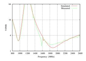
Fig. 3. *Three-band hybrid prefractal antenna* - Comparison between measured and simulated *VSWR* values.
